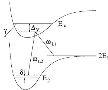
FIG. 1. Schematic diagram of the Raman photoassociation.
